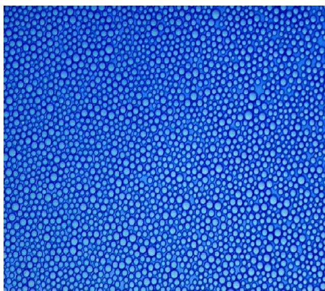
Fig. 8. Monodispersed emulsion formed with micro-fabricated microchannel array.
